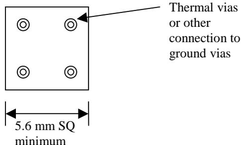
More information on this package and other requirements for using thermal lands and thermal vias are detailed in the TI application note *PowerPAD Thermally Enhanced Package Application*
