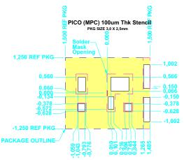
Figure 10. Pico (MPC) –100um Stencil Thickness Recommended Layout Target Solder Thickness after Reflow – Die = 50um (25/25um by Dome Print, On TAB = 30um)
