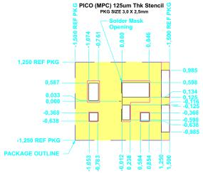
Figure 11. Pico (MPC) –125um Stencil Thickness Recommended Layout Target Solder Thickness after Reflow – Die = 63um (25/38um by Dome Print, On TAB = 43um)
