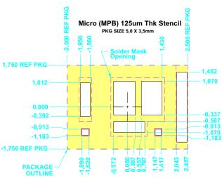
Figure 6. Micro (MPB) – 125µm Stencil Thickness Recommended Layout Target Solder Thickness after Reflow – Die = 63µm (25/38µm by Dome Print, On TAB = 43µm)
