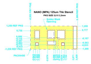
Figure 9. Nano (MPA) –125um Stencil Thickness Recommended Layout Target Solder Thickness after Reflow – Die = 63um
