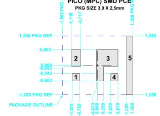
Figure 4. Pico (MPC) - Solder Mask Defined PCB Recommended Layout
