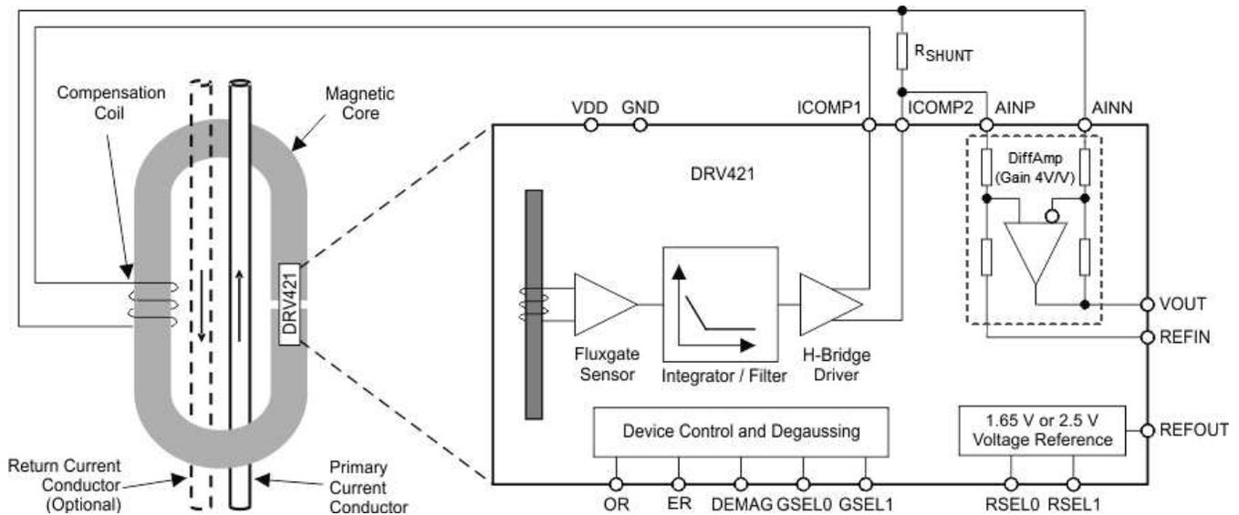
**Figure 1. Closed-Loop Current Sensor Module**
