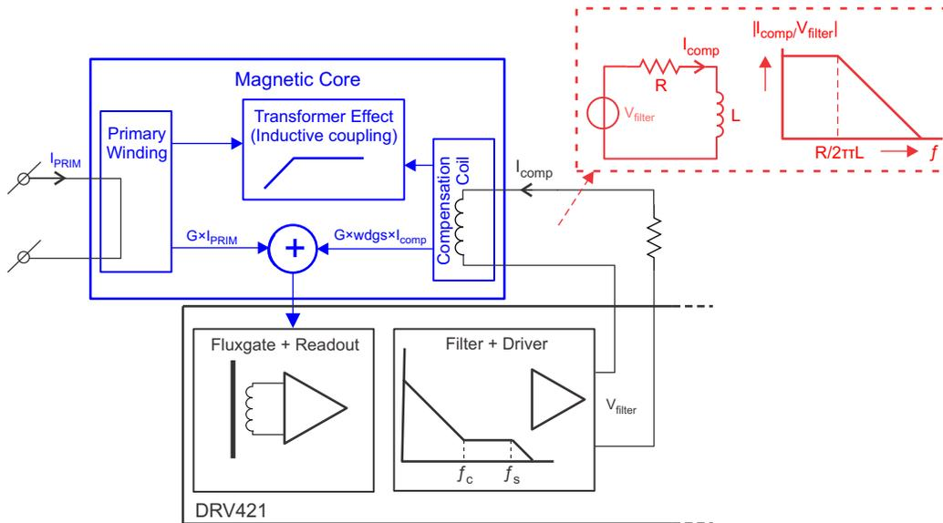
Figure 2. Current-Sensing Control Loop Comprising DRV421 and Magnetic Core
