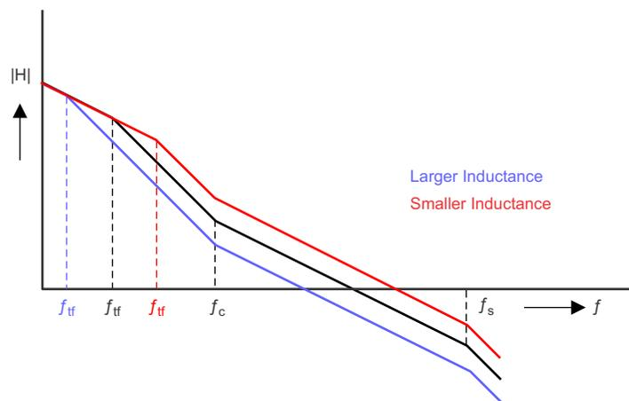
Figure 4. Effect of Inductance Change on Zero Crossing Frequency
