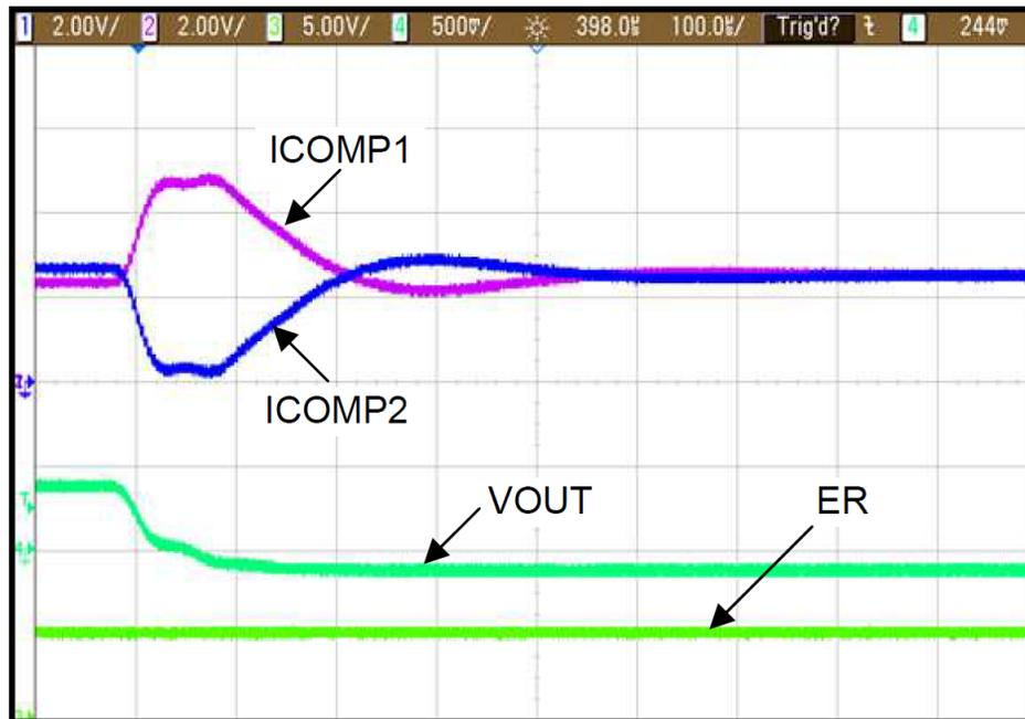
Figure 5. Settling of ICOMP1 and ICOMP2 with GSEL[1:0] = 10
