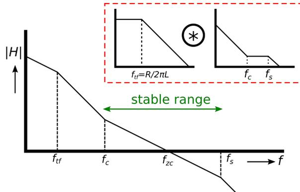
Figure 3. Bode Diagram of the Current-Sensing Loop
