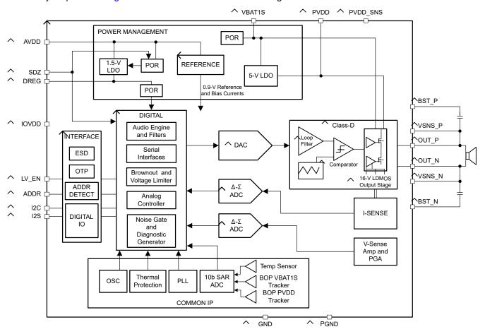
Figure 2-1. Functional Block Diagram
