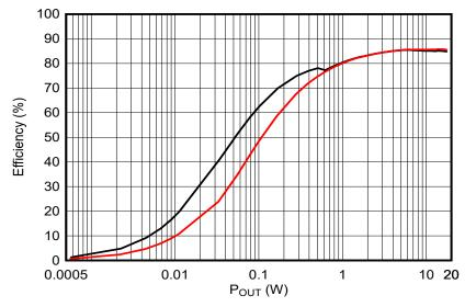
Figure 1-1. Efficiency Improvement by Using Y Bridge
