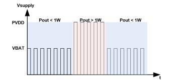
Figure 5-1. Y-Bridge Modulation
