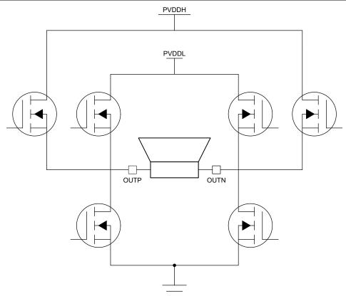
Figure 2-2. Simplified Y-Bridge Schematic
