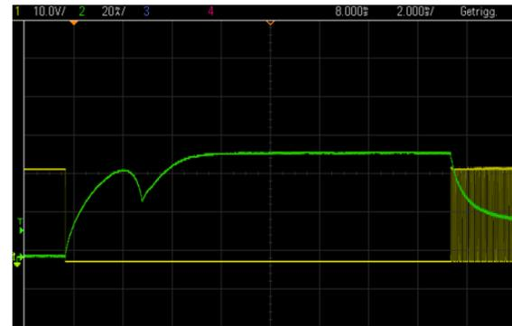
**Figure 2. Current and Voltage Controlling Magnetic Value**
