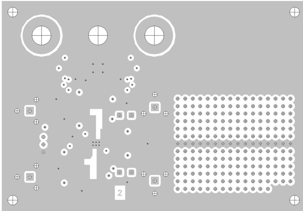
Figure 5–3. Internal Plane (Layer 3)
