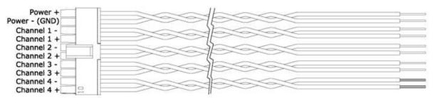
Figure 3. Wiring Harness for Power and Speaker Connections
