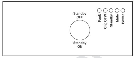
Figure 2. Front Panel Labels
