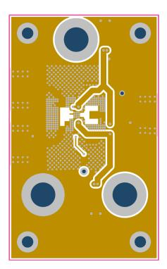
Figure 7. Layer 4 - GND/Signal
