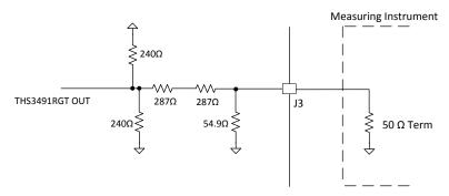
Figure 2. Output Interface to the Measuring Instrument
