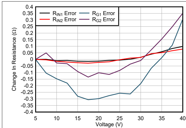
Figure 7-9. Resistor Actual-to-expected Mismatch vs Divider Voltage, Absolute
