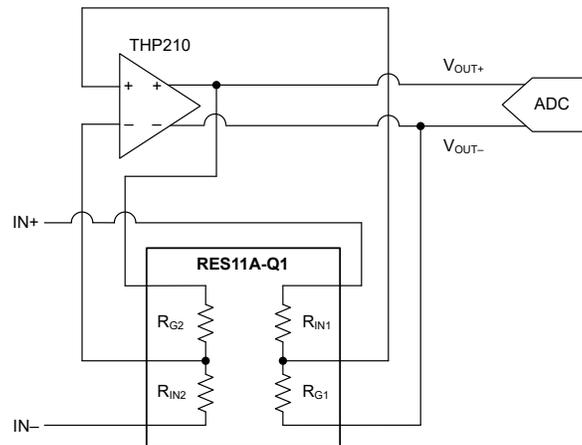
**Figure 8. Fully-Differential Amplifier Configuration**
