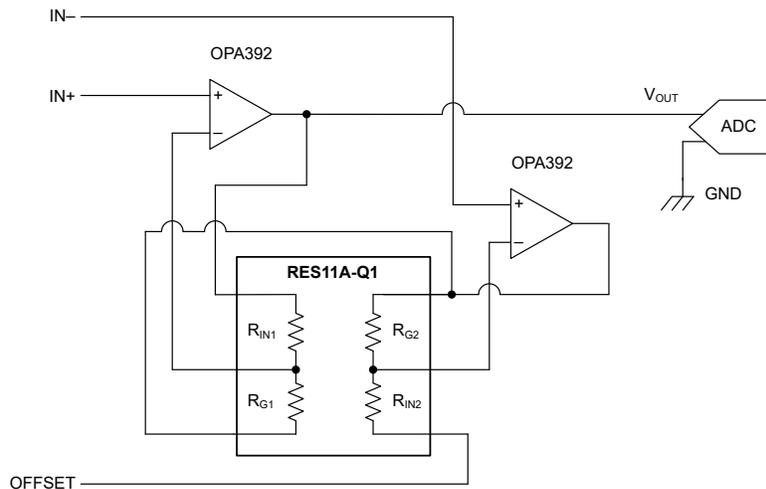
**Figure 7. Instrumentation Amplifier Configuration With Reference Input**
