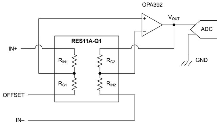
**Figure 5. Difference Amplifier Configuration**
