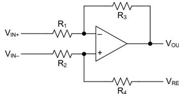
**Figure 4. Standard Differential Amplifier**
