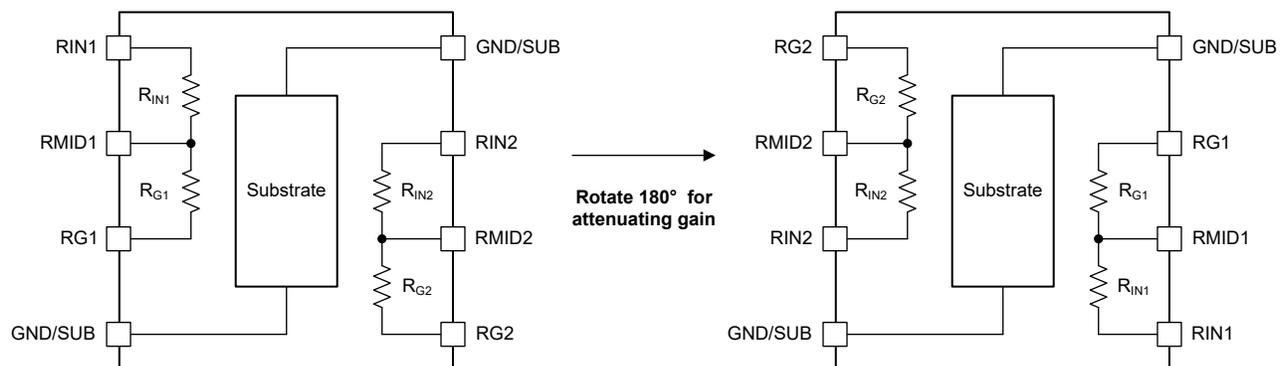
**Figure 3. Attenuating Gain Configuration**
