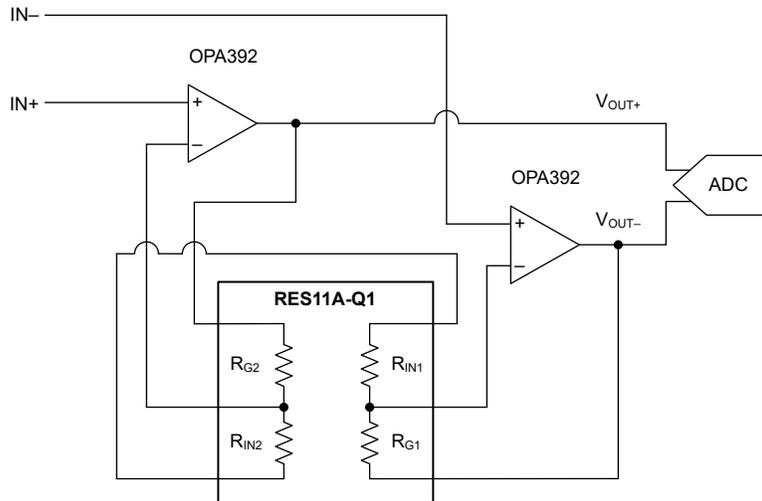
**Figure 6. Instrumentation Amplifier Configuration With Differential Output**
