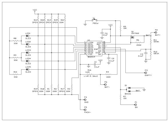
Figure 4. bq2014 Li-Ion Battery Capacity Monitoring System
