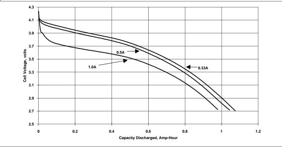
Figure 1. Li-Ion Battery Discharge Curve (Coke Electrodes)
