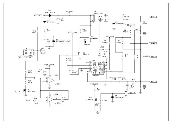
Figure 2. Li-Ion/NiMH bq2004 Switch-Mode Charging System
