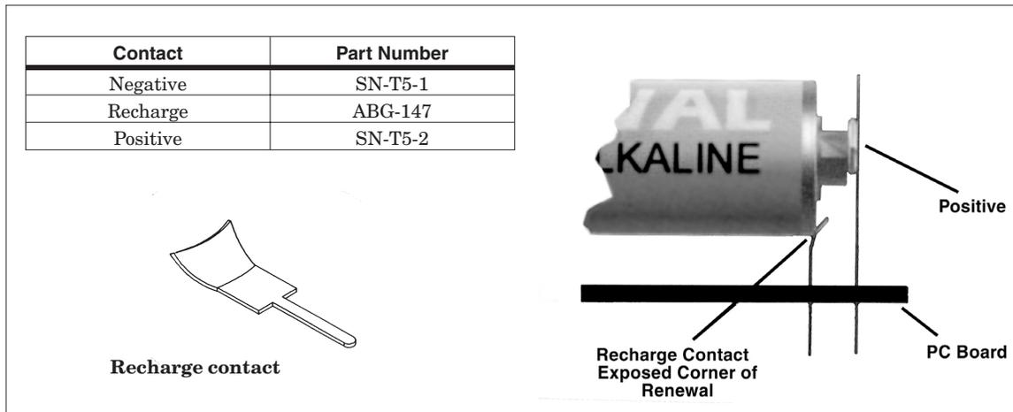
Figure 9. Charging Contacts for AA and AAA Cells
