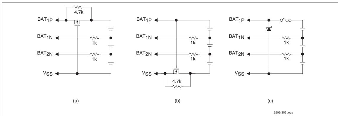
Figure 12. Protecting the bq2902/3 Against Reverse Battery Insertion
