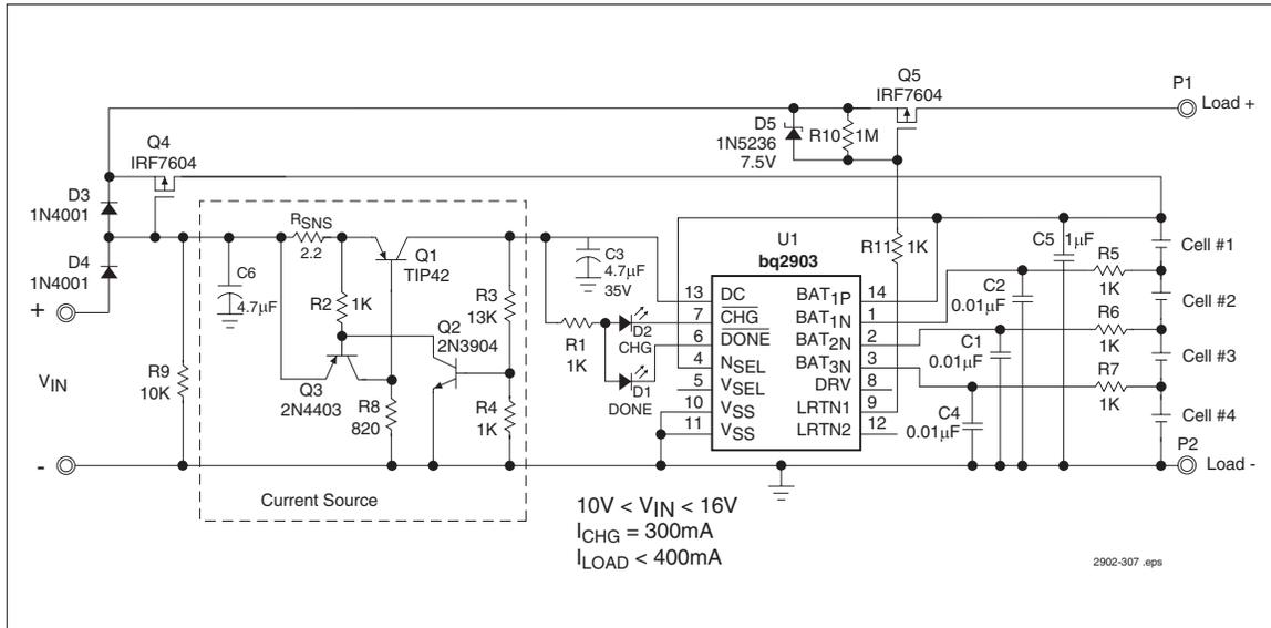
**Figure 7. Discharge Control With High-Side Load Switch**
