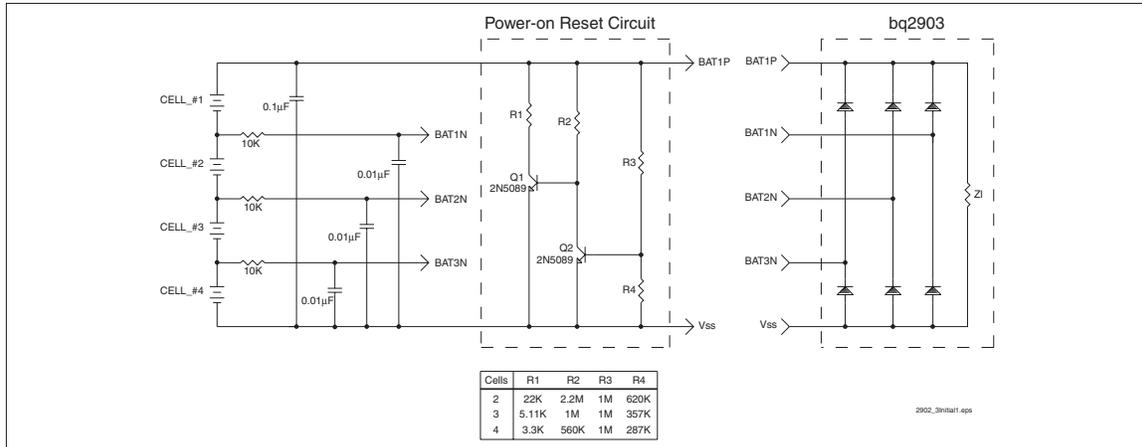
Figure 11. Automatic Power-Up Initialization
