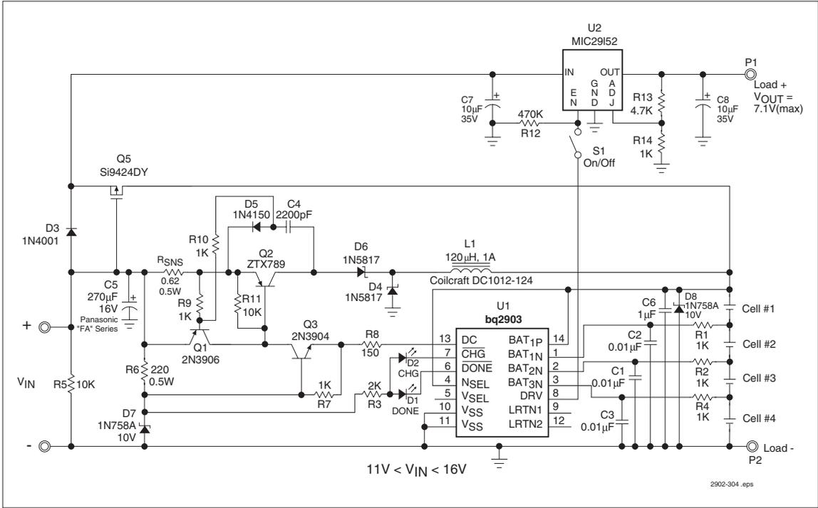
**Figure 6. One-Amp Switch-Mode Charger Using an LDO for a Voltage Clamp and High-Side Load Switch**
