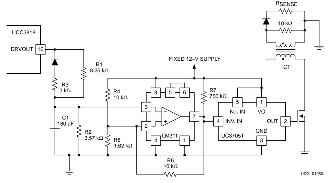
Figure 1. Maximum Duty Cycle Clamp Application
