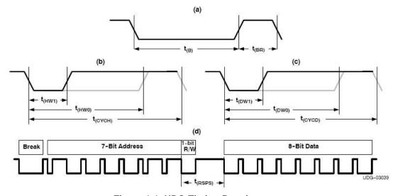
Figure 1-1. HDQ Timing Requirements
