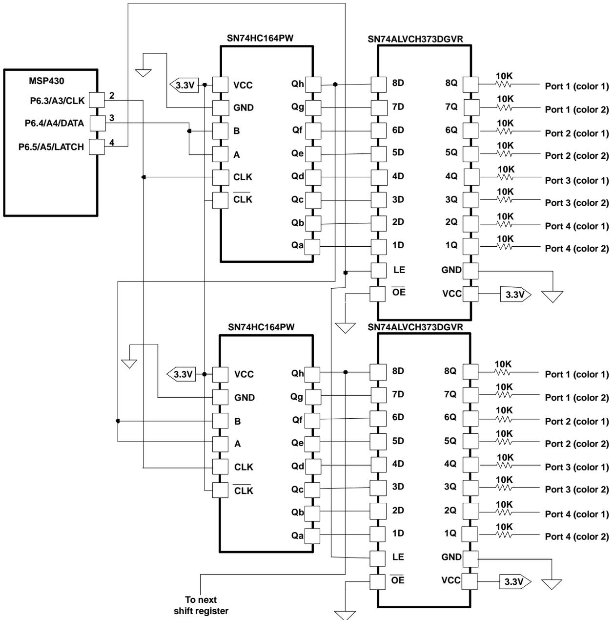
Figure 6. LED Interface Schematic
