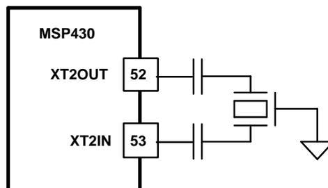
**Figure 8. Clock Circuit Interface**
