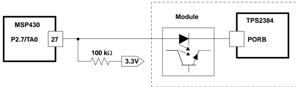
Figure 10. Power-On Reset Circuit Interface
