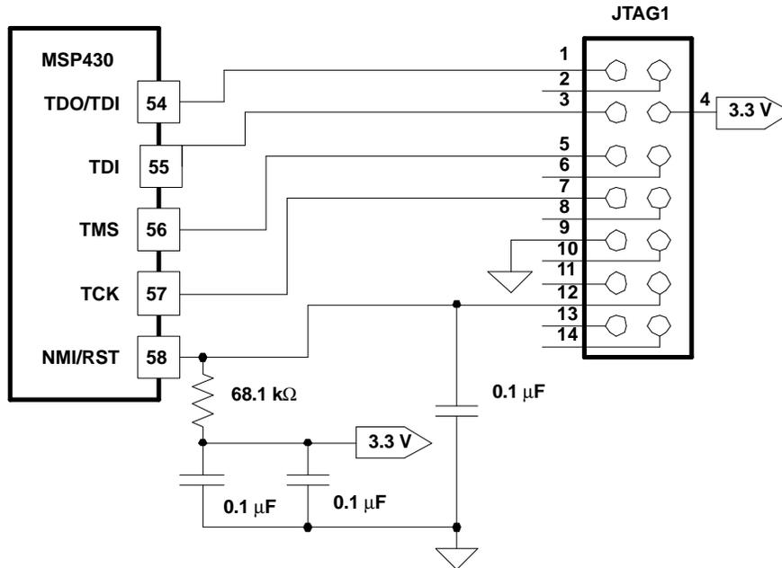
Figure 4. JTAG Interface Schematic
