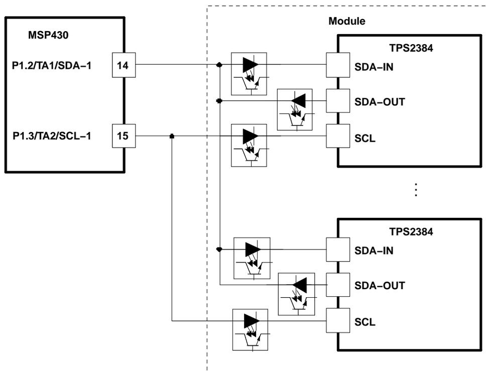
**Figure 3. PSE Communications Interface (I<sup>2</sup>C) Schematic**
