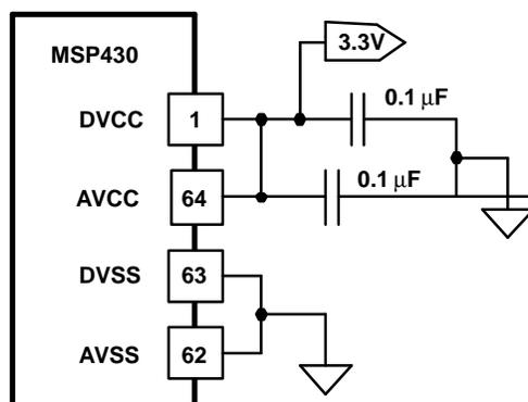
Figure 9. Power and Ground Schematic
