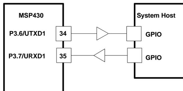
Figure 2. Host Communications Interface (RS-232) Schematic
