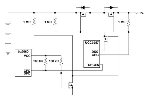
Figure 2. Using the CFC Pin to Control CHGEN on the UCC3957
