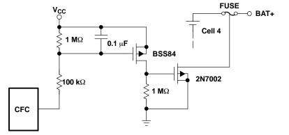
CFC and DFC Operation in the bg2060A Gas Gauge IC
