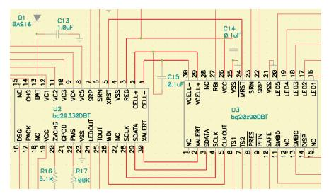
Figure 1. Orient the Chipset to Take Advantage of Easy Interconnection
