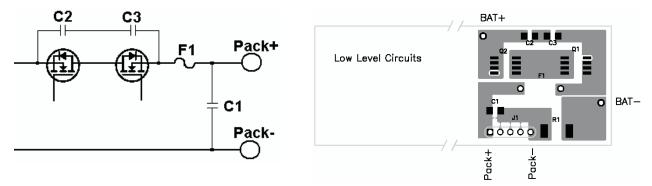
Figure 5. Use Wide Copper Traces to Lower the Inductance of Bypass Capacitors C1, C2, and C3
