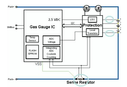
Figure 8. Correct: In Some Cases, Top and Bottom Cell Voltage Sensing May Be Extended Out to Cells
