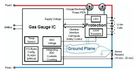
Figure 6. ICs Use a Low-Current Ground System. Ground Plane is Optional.
