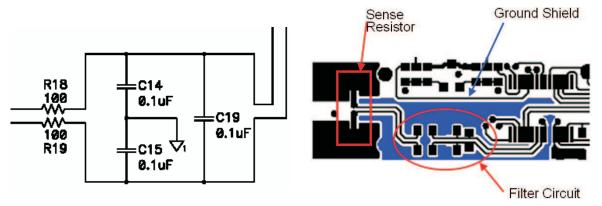
Figure 9. Differential Filter Components With Symmetrical Layout
