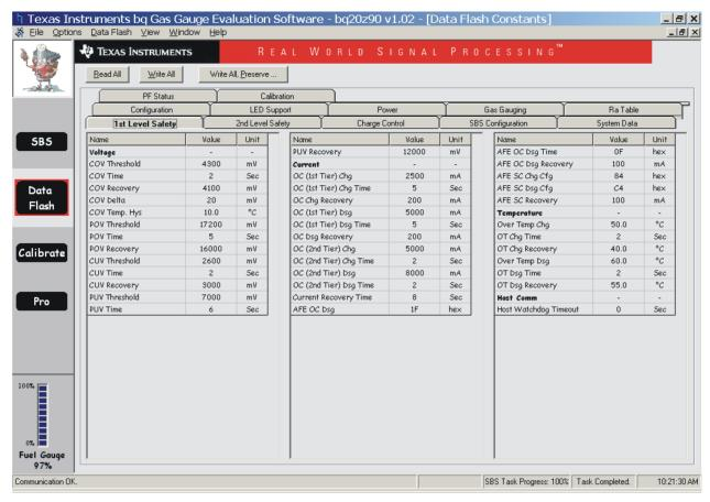
Figure 4. Example of bq20z70/90 Data Flash Organization. 1st Level Safety Class of Data Flash Constants. Subclasses are Voltage, Current, Temperature, and Host Comm.
