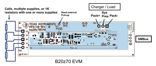
Figure 1. bg20z90 EVM Connections
