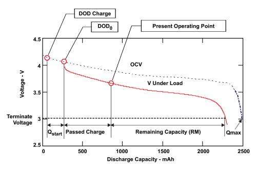
Figure 3. OCV Characteristics (Dotted Curve) and Battery Discharge Curve Under Load (Solid Curve)
