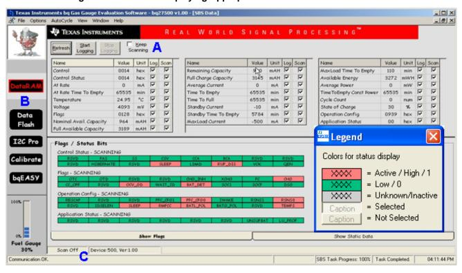
Figure 10. DataRAM Displaying Appropriate Communication with EV2300
