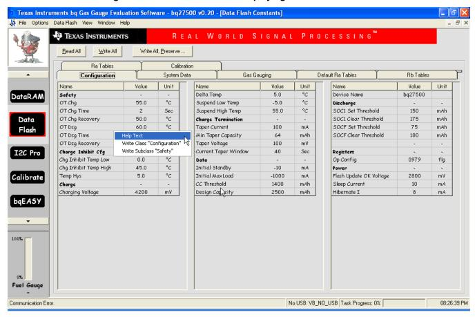
Figure 11. Data Flash Window Displaying Default Parameters
