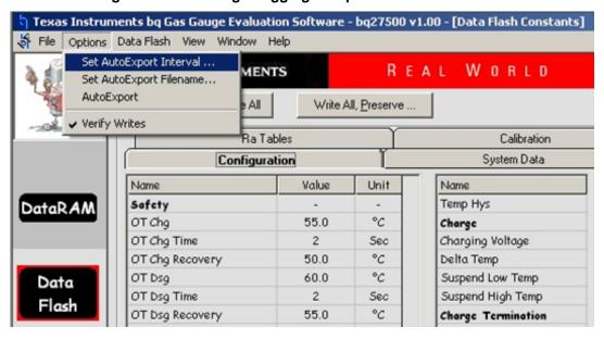
Figure 21. Gas Gauge Logging Setup and Start Commands
