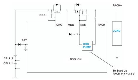
Figure 2. Simplified Drawing of Gate Drive Circuit for Discharge FET
