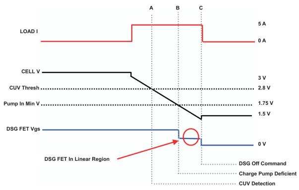
Figure 4. Abnormal Cell Undervoltage Protection
