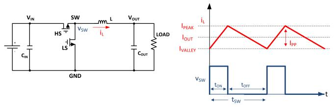
Figure 2-1. Basic synchronous buck regulator and waveforms
