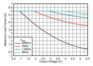
Figure 4-1. Ideal Maximum Load Current Due to HS Current Limit Only (V<sub>IN</sub> = 12 V, L = 470 nH)
