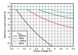
Figure 4-2. Maximum Load Current Due to HS Current Limit Only (V<sub>IN</sub> = 12 V, L = 325 nH (70% of Nominal))
