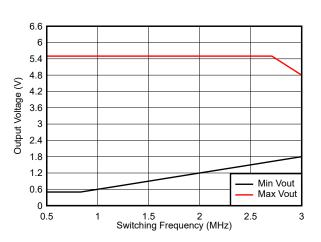
Figure 3-1. TPSM5D1806 Output Voltage Range Due to Minimum On- and Off-Time Only (V<sub>IN</sub> = 12 V)
