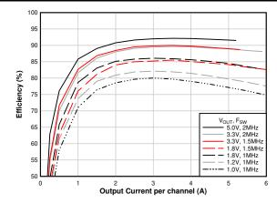
Figure 4-5. TPSM5D1806 Efficiency vs Output Current (V<sub>IN</sub> = 12 V)
