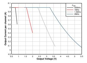
Figure 5-1. TPSM5D1806 Maximum Output Current (V<sub>IN</sub> = 12 V)
