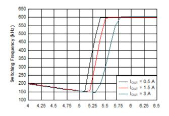
Figure 3-5. Frequency Foldback at Dropout (V<sub>OUT</sub> = 5 V)
