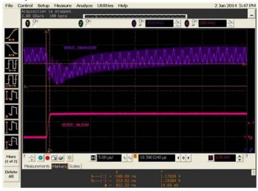
Figure 4-1. Step-Up Load Transient Response
