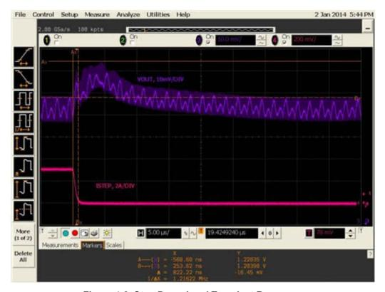
Figure 4-2. Step-Down Load Transient Response
