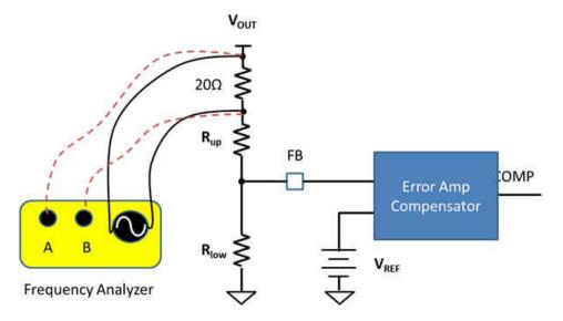
Figure 1-1. Voltage-Mode or Current-Mode Control-Loop Gain Setup
