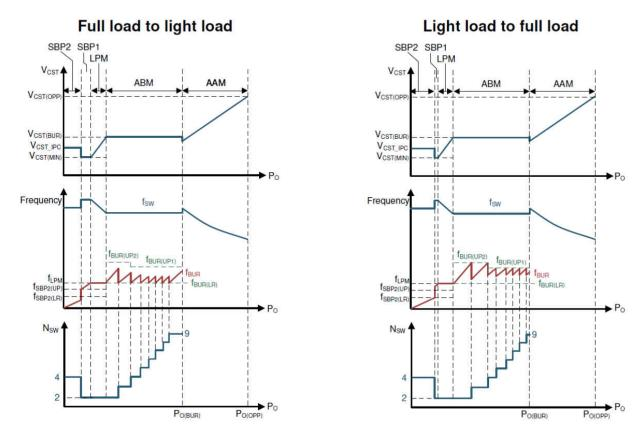
Figure 2-2. Control Law Under Different Load Sweep Direction as  $V_{IPC} > 0.9$  V and  $V_{VS} > V_{VSLV(UP)}$
