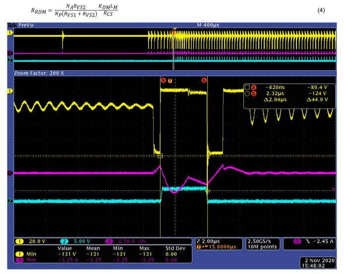
Figure 4-2. SR VDS spike during first high side turn on
