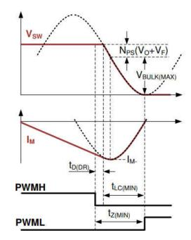
Figure 4-3. RTZ Setting for the Falling-edge Transition of VSW
