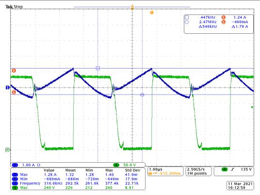
Figure 4-4. RTZ Setting too large cause VDS ring back
