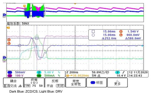
Figure 4-5. UCC28056 Triggers O<sub>CP2</sub> Protection
