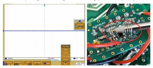
Figure 3-1. Fine Scale Menu of the Oscilloscope and Probe Connecting
