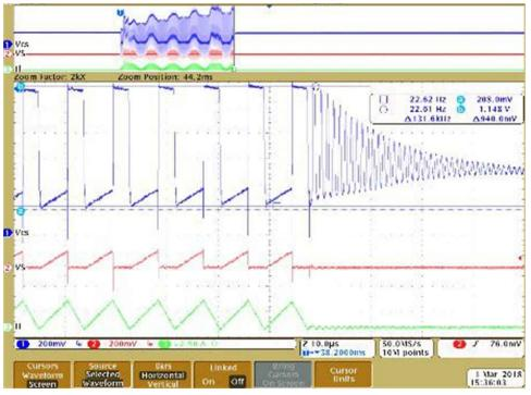
Green: PFC inductor current, Blue: ZCD/CS, Red: Voltage on current sense resistor
