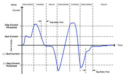
Figure 4-1. Gauge Operating Mode
