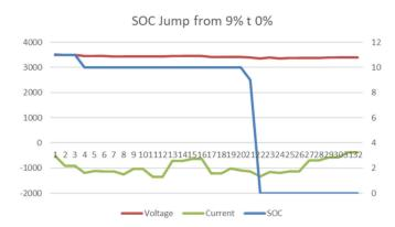
Figure 7-1. SOC Jump From 9% to 0%
