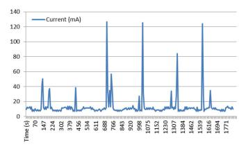
Figure 4-2. Power Consumption When the Phone Is In Idle State
