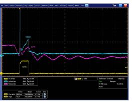
CS signal starts at 0 V, slope of the CS follows Rsense
