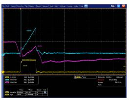
CS signal starts below 0 V, slope of CS does not follow Rsense
