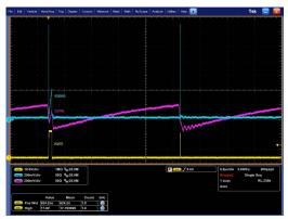
Inconsistent gate pulse widths
