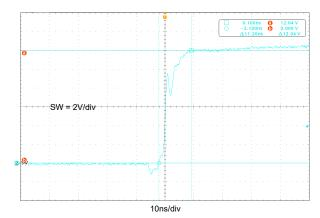
Figure 5-7. EVM Board with TPS565242 Switching Spike,  $V_{IN} = 12 \text{ V}$ ,  $V_{OUT} = 1.05 \text{ V}$ ,  $I_{OUT} = 5 \text{ A}$
