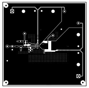
Figure 5-1. Co-layout Design Top Layer
