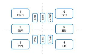
Figure 4-2. Type 2 - Piggyback Co-layout for TPS56x201/8 and TPS56x242/7
