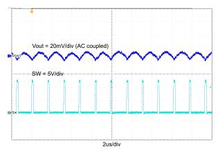
Figure 5-3. EVM Board with TPS565242 Output Ripple,  $V_{IN} = 12 \text{ V}$ ,  $V_{OUT} = 1.05 \text{ V}$ ,  $I_{OUT} = 5 \text{ A}$
