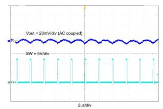
Figure 5-5. EVM Board with TPS565201 Output Ripple,  $V_{\text{IN}}$  = 12 V,  $V_{\text{OUT}}$  = 1.05 V,  $I_{\text{OUT}}$  = 5 A
