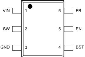
Figure 2-3. TPS56x202/3/6/7 Pin-out
