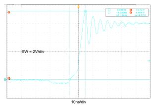
Figure 5-10. Co-layout Board with TPS565201 Switching Spike,  $V_{IN}$  = 12 V,  $V_{OUT}$  = 1.05 V,  $I_{OUT}$  =
