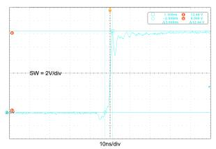
Figure 5-8. Co-layout Board with TPS565242 Switching Spike,  $V_{IN}$  = 12 V,  $V_{OUT}$  = 1.05 V,  $I_{OUT}$  =
