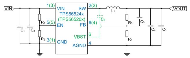
Figure 3-1. Schematic Diagram to Achieve Co-lay
