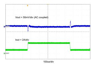
Figure 5-13. Co-layout Board with TPS565201 Transient Response,  $V_{IN}$  = 12 V,  $V_{OUT}$  = 1.05 V, 0.1 A Transient Response,  $V_{IN}$  = 12 V,  $V_{OUT}$  = 1.05 V, 1.25 - 2.5 A
