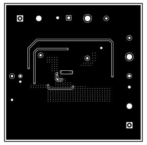
Figure 5-2. Co-layout Design Bottom Layer
