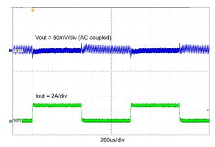
Figure 5-11. Co-layout Board with TPS565242 Transient Response,  $V_{IN}$  = 12 V,  $V_{OUT}$  = 1.05 V, 0.1 A Transient Response,  $V_{IN}$  = 12 V,  $V_{OUT}$  = 1.05 V, 1.25
