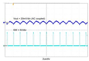
Figure 5-4. Co-layout Board with TPS565242 Output Ripple,  $V_{IN} = 12 \text{ V}$ ,  $V_{OUT} = 1.05 \text{ V}$ ,  $I_{OUT} = 5$
