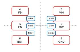
Figure 4-1. Type 1 - Mirror Symmetrical Co-layout for TPS56x201/8 and TPS56x202/3/6/7
