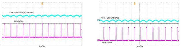
Figure 4-1. TPS564242 12V Input to 1.05V Output at Figure 4-2. TPS563203 12V Input to 1.05V Output at 4A 3A
