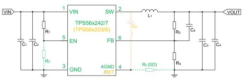
Figure 3-4. Co-Layout Schematic for TPS56x242/7 and TPS56x203/6
