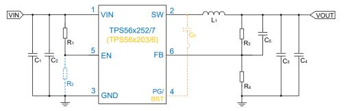
Figure 3-3. Co-layout Schematic for TPS56x252/7 and TPS56x203/6
