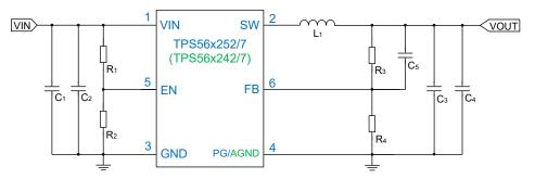
Figure 3-2. Co-Layout Schematic for TPS56x252/7 and TPS56x242/7
