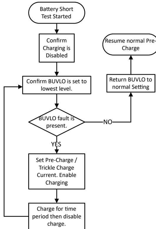
**Figure 2-2. Short Test Flow**
