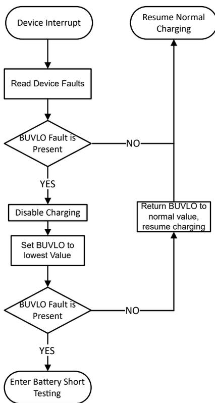
**Figure 2-1. Battery Monitoring Flow**
