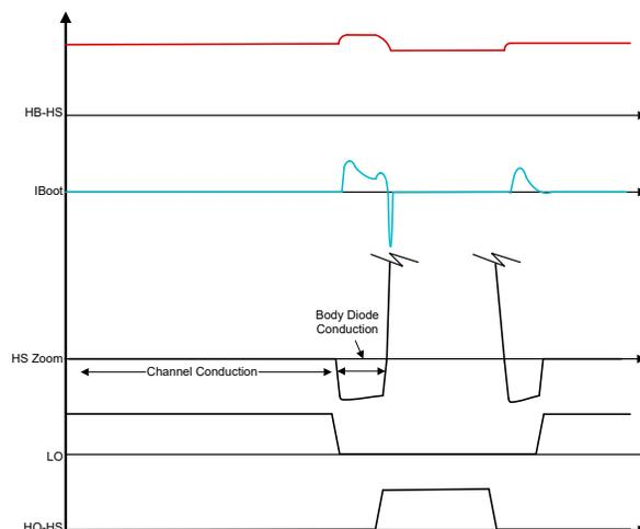
Figure 4-1. Detail Timing Diagram of Steady State HS Voltage and Boot Diode Current
