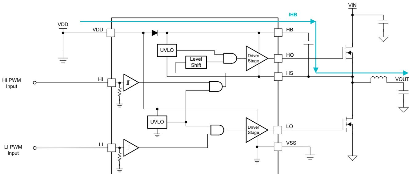
**Figure 1-1. Simplified Synchronous Buck Showing Boot Capacitor Charging Path**
