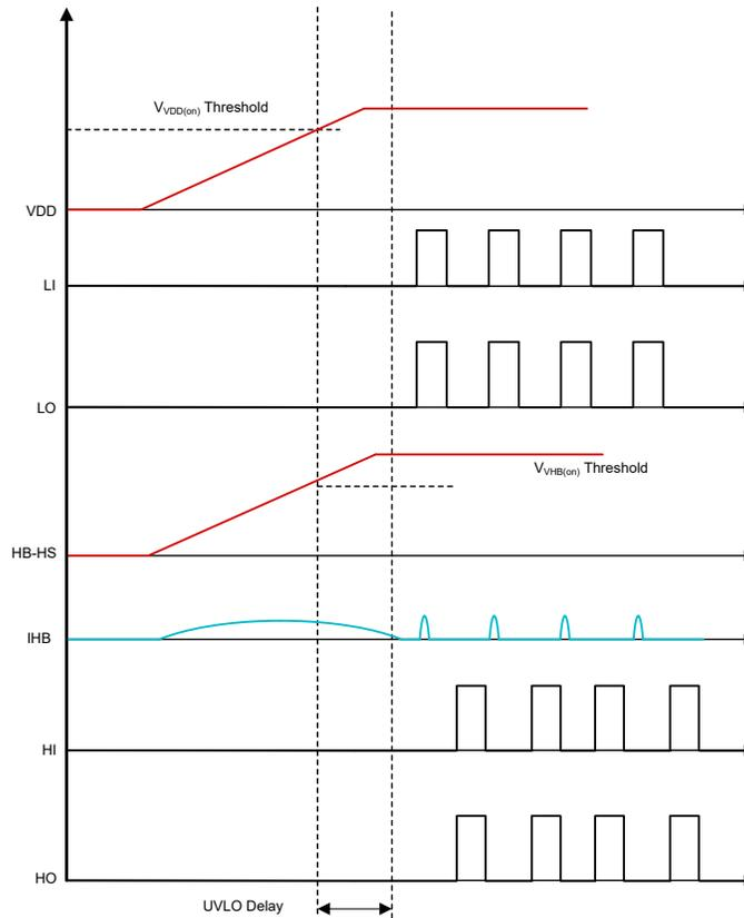
**Figure 1-2. Synchronous Buck Timing Diagram**
