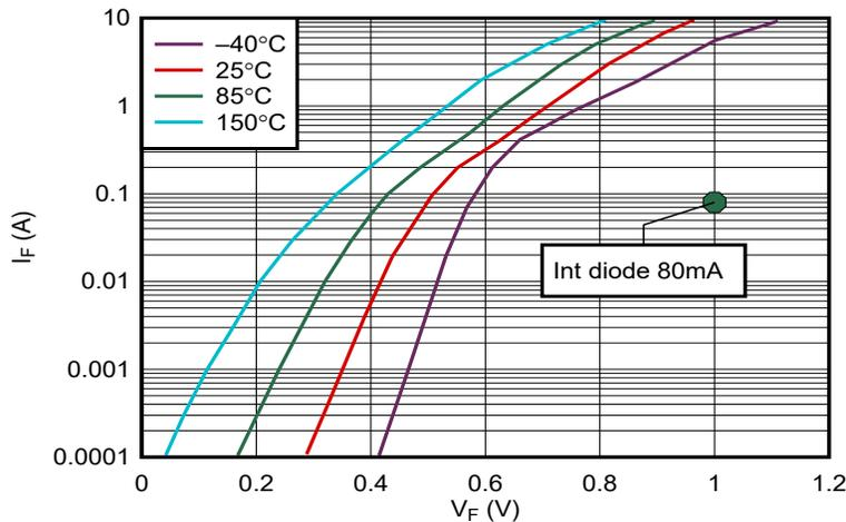
Figure 3-1.  $V_F$  Vs  $I_F$  of Example External Boot Diode
