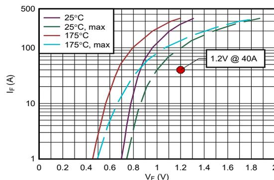
Figure 5-1. Power MOSFET Example Body Diode  $V_F$  Vs  $I_F$
