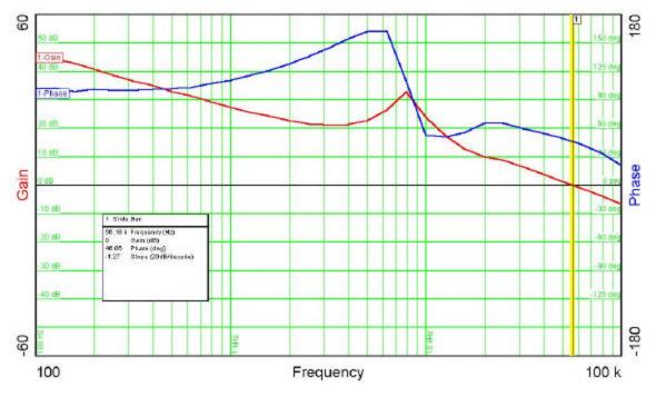
The plot below shows the loop gain and phase margin with output voltage set to 5V. The output shows all 3 variations on one graph.
