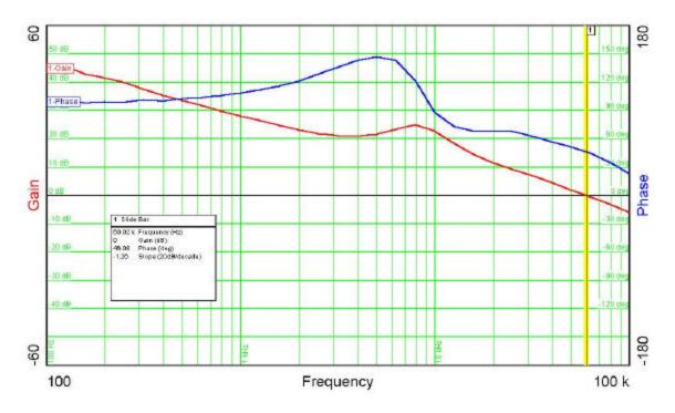
The plot below shows the loop gain and phase margin with output voltage set to 5V. The output was loaded to 3A. Vin = 12V
