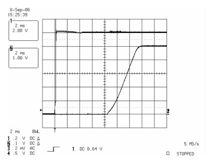
The photo below shows the 5V output voltage (Ch2) startup waveform after the application of 12Vdc in (Ch1). The output was loaded to 3A.
