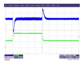
5V transient response with a 24V input and a load step from 125mA to 250mA on the 3.3V output:
