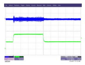
3.3V transient response with a 24V input and a load step from 125mA to 250mA on the 3.3V output:
