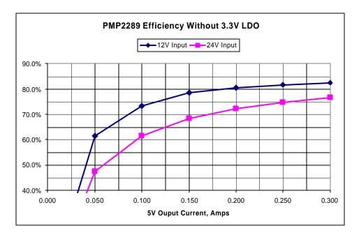
The efficiency versus input voltage is shown below. The 5V output is loaded to 50mA.
