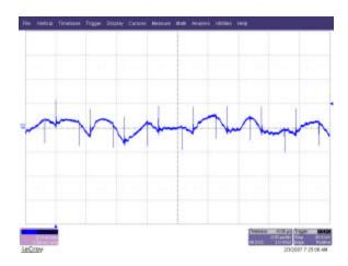
5V output voltage ripple with a 24V input and loads of 5V/50mA; 3.3V/250mA:
