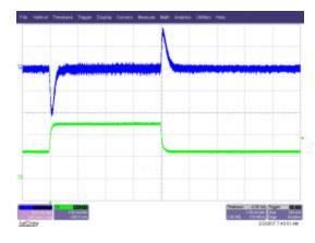
3.3V transient response with a 12V input and a load step from 125mA to 250mA on the 3.3V output:
