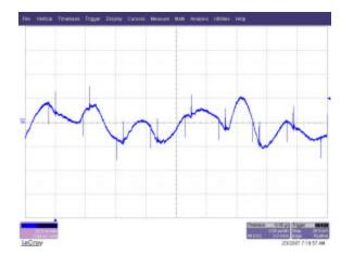
3.3V output voltage ripple with a 12V input and loads of 5V/50mA; 3.3V/250mA:
