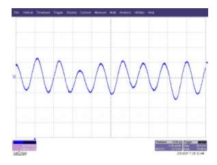
3.3V output voltage ripple with a 24V input and loads of 5V/50mA; 3.3V/250mA:
