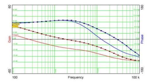
The figure below is the loop gain of the flyback converter with a 24V input. The marked gain/phase is with a 300mA load on the 5V. The unmarked gain/phase is with a 50mA load on the 5V.
