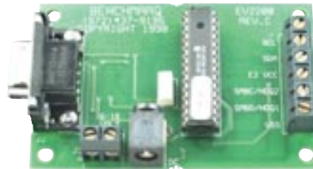
The EV2200 PC-interface board allows the PC to talk to the gas gauge IC using the PC serial port.
