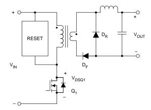
Fig. 1. Forward converter with diode rectification.
