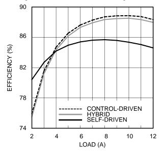
Fig. 26. Efficiency vs. load current.
