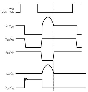
*Fig. 9. Control-driven synchronous rectification waveforms.*
