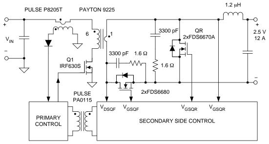
Fig. 17. Simplified prototype schematic.
