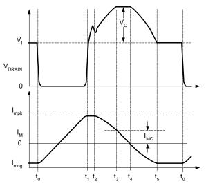
Fig. 3. Primary MOSFET  $Q_1$  drain-to-source voltage and the transformer magnetizing current for an R-C-D clamp forward converter.
