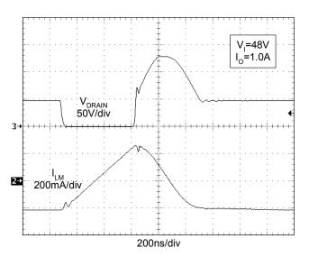
Fig. 4. Primary MOSFET Q1 drain-to-source voltage and transformer magnetizing current.
