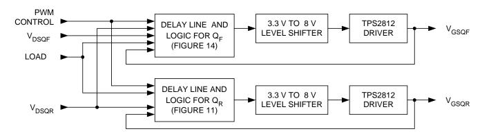
Fig. 18. Secondary side control block diagram.
