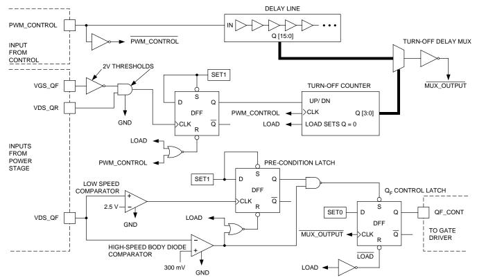
Fig. 14.  $Q_F$  control circuitry.
