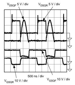
*Fig. 21. Control-driven synchronous rectification waveforms.*
