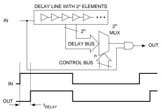
Fig. 10. Delay block.
