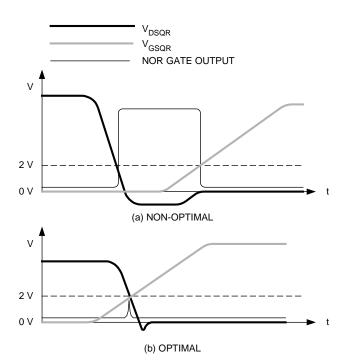
Fig. 12.  $Q_R$  turn-on waveforms.
