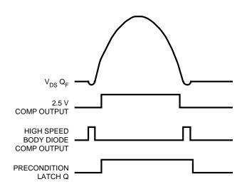
Fig. 15.  $Q_F$  pre-condition latch waveforms.
