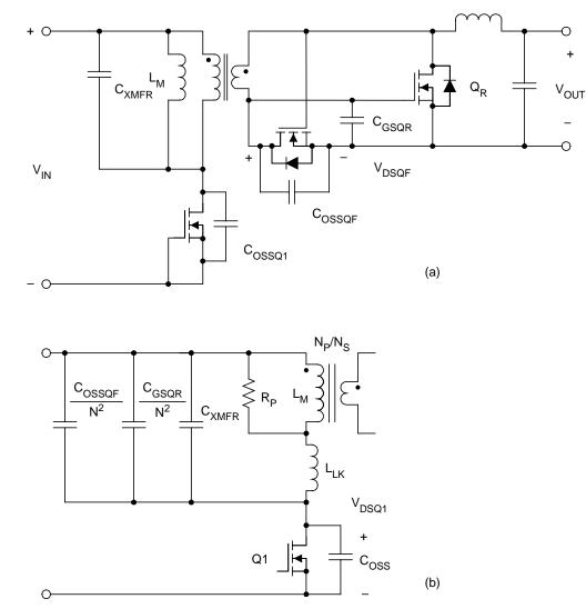
Fig. 8. Capacitances of the resonant circuit (a) and equivalent resonant capacitances and inductance reflected to the primary side (b).
