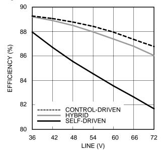
Fig. 27. Efficiency vs. input line voltage.
