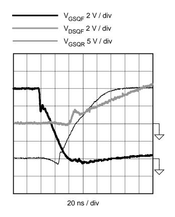
Fig. 25.  $Q_F$  turn-off waveforms.
