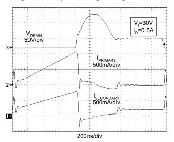
Fig. 5. Primary MOSFET Q1 drain-to-source voltage and transformer primary and secondary currents.
