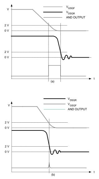
Fig. 16. Q<sub>F</sub> turn-off waveforms.
