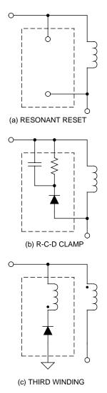
Fig. 2. Possible reset mechanisms.
