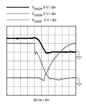
Fig. 22. $Q_R$  turn-on waveforms.
