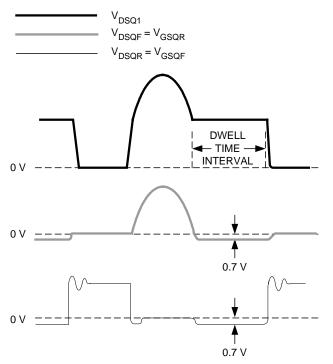
*Fig. 7. Typical waveforms for self-driven synchronous forward converters with resonant reset.*
