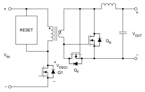
Fig. 6. Forward converter with self-driven synchronous rectifiers.
