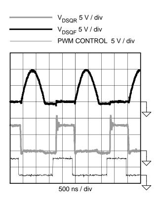
Fig. 20. Self-driven synchronous rectification waveforms.
