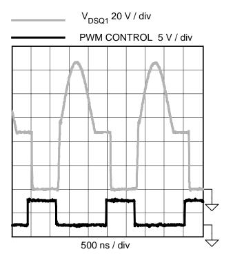
Fig. 19. Resonant reset waveforms.
