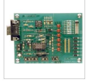
The menu-driven software provided with the EV2012 displays charge/discharge activity and allows user interface to the bq2012 from any standard DOS PC.
