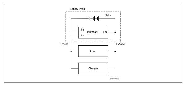
Figure 1. Module Connection Diagram
