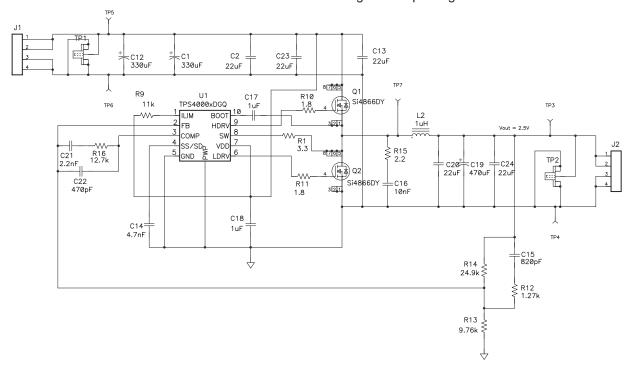
Figure 1. Application Diagram for the TPS40000/1
