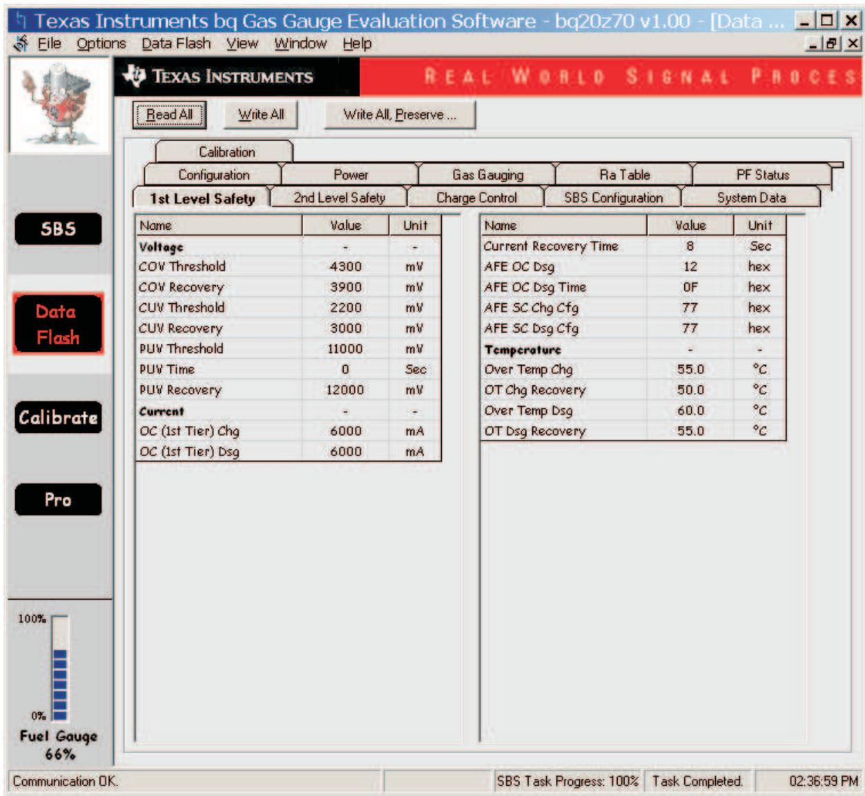
Figure 9. Data Flash Screen, 1st Level Safety Class
