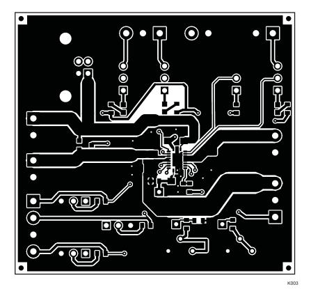
Figure 5. Board Layout - Top Etch Layer
