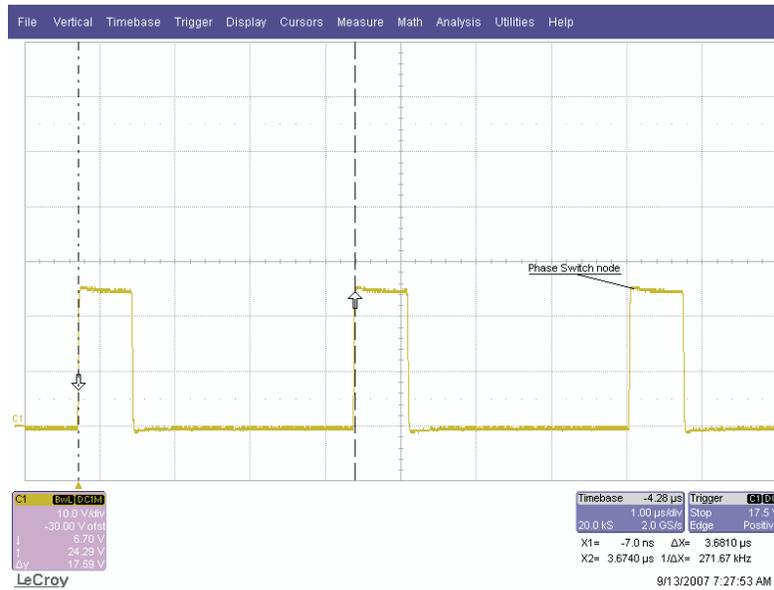
**Figure 3. Phase Switching Node of DC-DC Converter**
