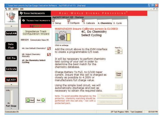
Figure 18. Chemistry Cycling Test
