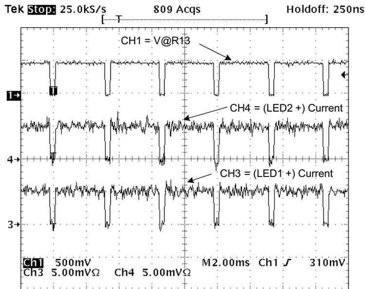
Figure 13. Current LED1 (CH3) and LED2 (CH4)
