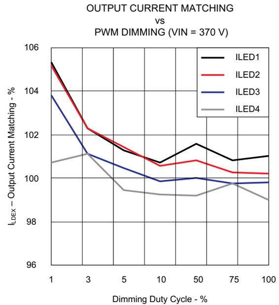
Figure 6.  $V_{IN} = 370\text{ V}$ , Current Matching
