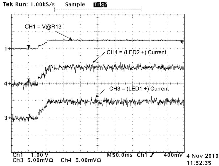
Figure 11. Current LED1 (CH3) and LED2 (CH4)
