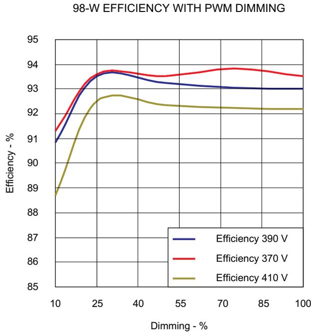
Figure 8. Efficiency 10% to 100% PWM Dimming
