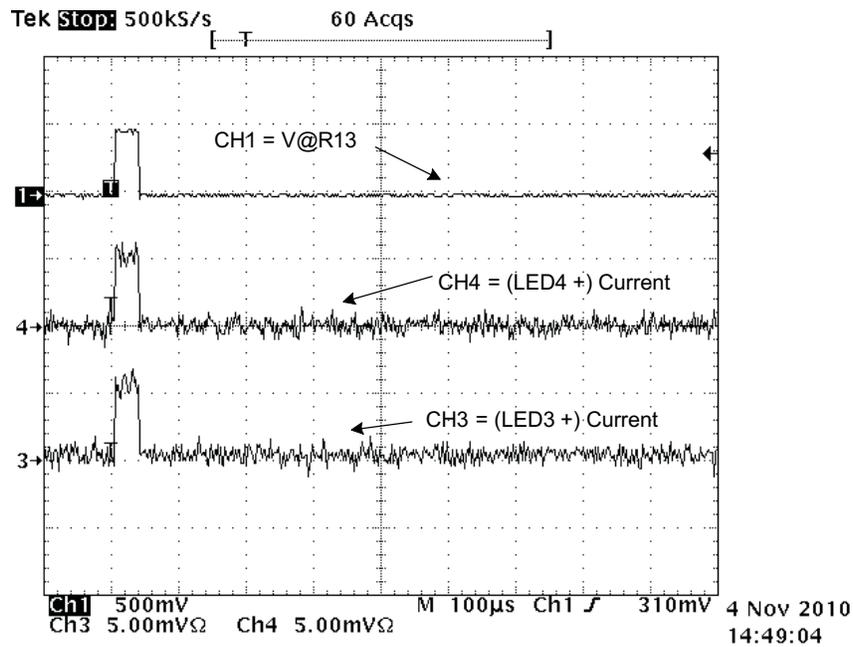
Figure 16. Current LED3 (CH3) and LED4 (CH4)
