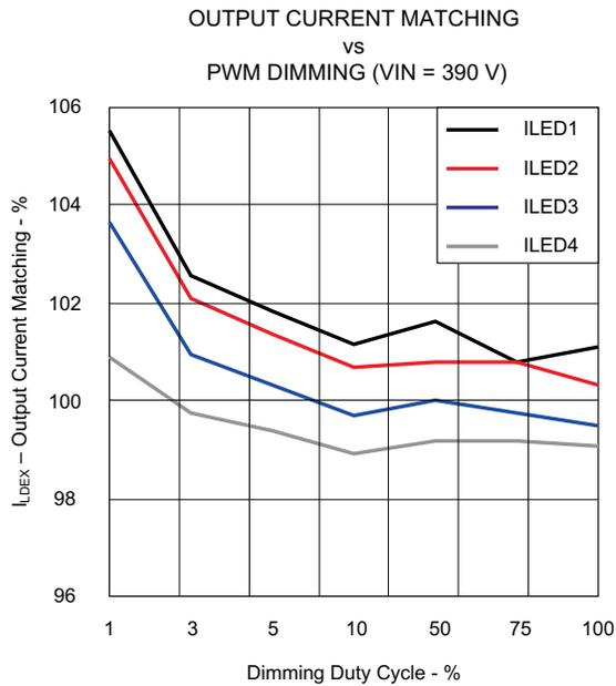
Figure 5.  $V_{IN} = 390\text{ V}$ , Current Matching
