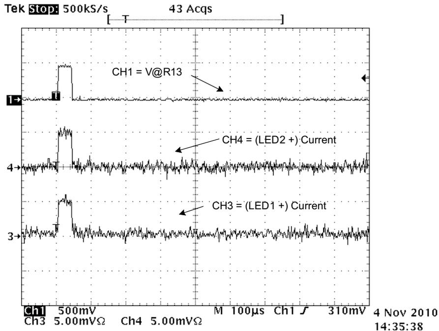
Figure 15. Current LED1 (CH3) and LED2 (CH4)
