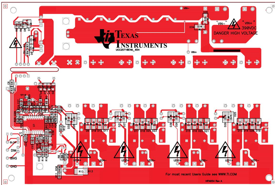
Figure 18. Bottom Assembly/Layout
