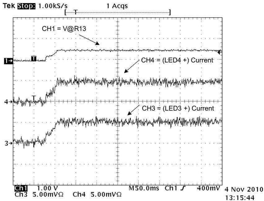
Figure 12. Current LED3 (CH3) and LED4 (CH4)
