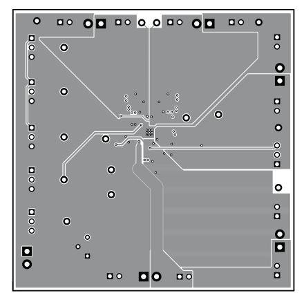
Figure 7. First Internal Layer
