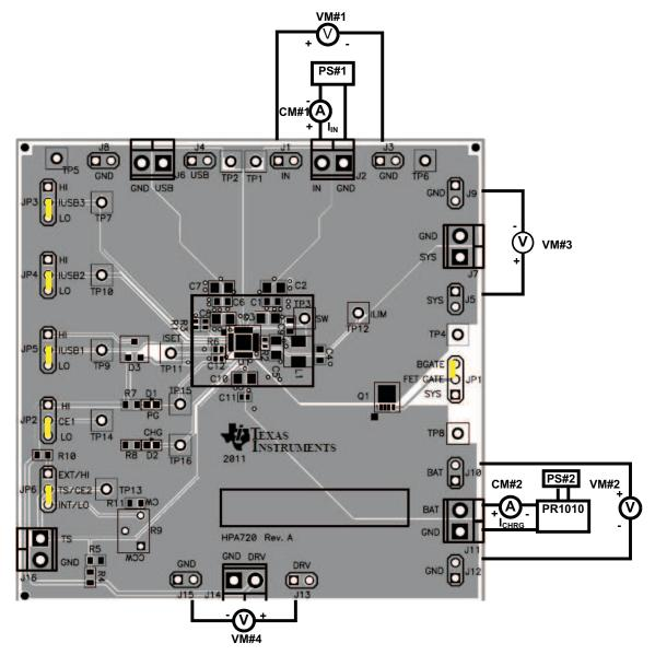
Figure 3. Original Test Setup for bq24165/166/167EVM (HPA720)
