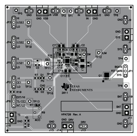
Figure 4. Top Assembly Layer
