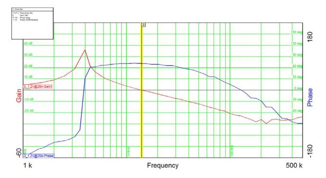
$\begin{array}{lll} \text{Input voltage} & = 13.5 \text{VDC} \\ \text{Output voltage} & = 1.2 \text{V} \\ \text{Load current} & = 25 \text{A} \\ \text{Phase margin} & = 71.4^{\circ} \\ \text{Bandwidth} & = 14 \text{kHz} \end{array}$
