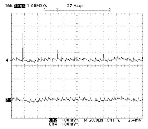
Figure 13. Output Ripple Voltage at Full Load
