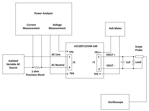
Figure 3. Test Setup
