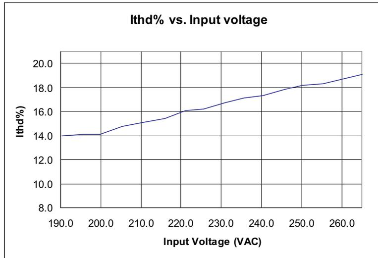
Figure 7. *I*<sub>thd</sub>% vs Input Voltage
