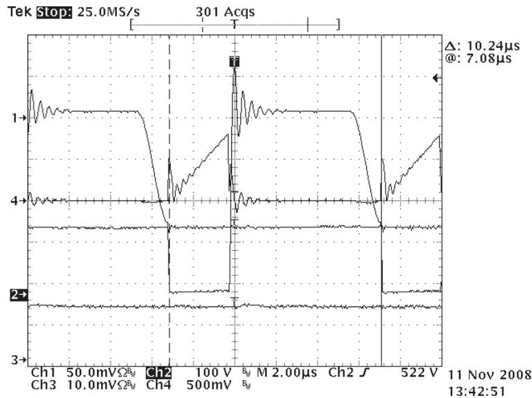
**Figure 12. Switch Frequency**
