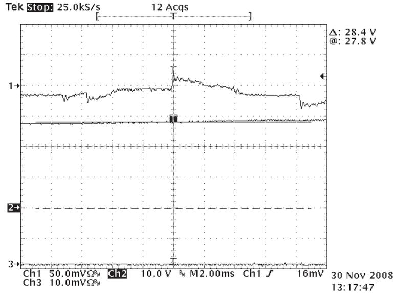
**Figure 15. LED Open Circuit Waveforms**
