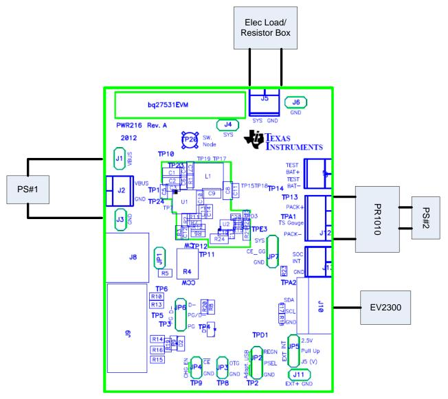
Figure 8. Test Setup for bq27531EVM (PWR216)
