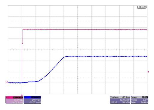
The photo below shows the 12V output voltage startup waveforms after the application of 48Vdc in. The output was loaded with a 1A resistive load. (Vin is 10V/DIV, Vout is 5V/DIV, 10mS/DIV)
