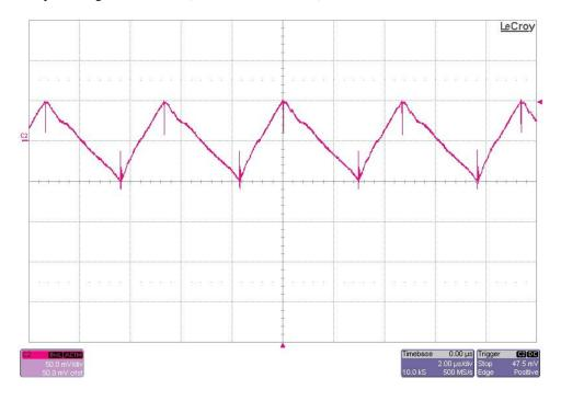
The 12V output ripple voltage is shown in the figure below. The image was taken with the output loaded to 1A and the input voltage set to 12Vdc. (50mV/DIV, 2uS/DIV)
