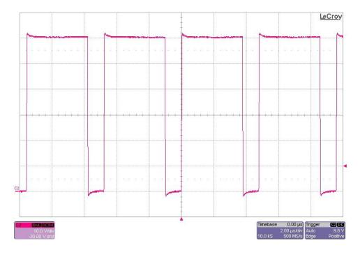
The photo below is the N-ch FET drain waveform. The input voltage is 48V and the output is loaded to 0.345A (the converter is entering discontinuous operation). (10V/DIV, 2uS/DIV)
