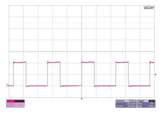
The photo below is the N-ch FET drain waveform. The input voltage is 8V and the output is loaded to 0.075A (the converter is entering discontinuous operation). (10V/DIV, 2uS/DIV)
